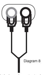
Typical speaker output using spade connectors. Insert bare wire into the binding post and tighten.
